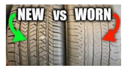
Tires are specifically designed with surfaces called treads. These treads are designed to form channels that push away water and snow to help tires maintain contact with the roadway surface. It is important to check and monitor the tread on your tires to make sure your tires are operating properly. Be on the lookout for thinning areas or smoothness which results in diminished traction.
